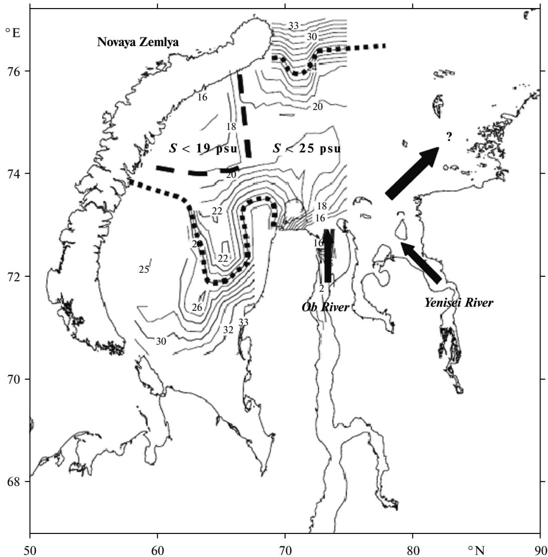
**Fig. 1.** Distribution of the salinity in the surface layer of the southwestern Kara Sea based on evidence derived from data of the CTD probe built into the flow-through system.
