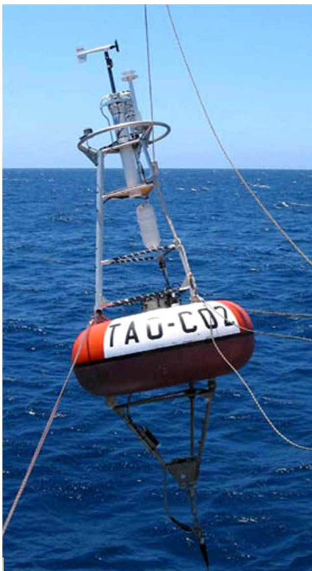
Figure 9. An example of a mooring with an autonomous pCO 2 sensor being deployed in the tropical Pacific.
