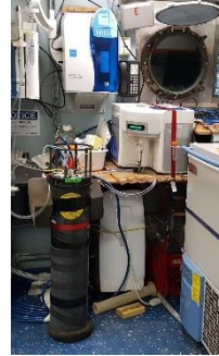
Underway flow cytometry and Imaging FlowCytobot
