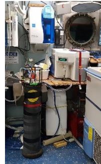
Underway flow cytometry and Imaging FlowCytobot
