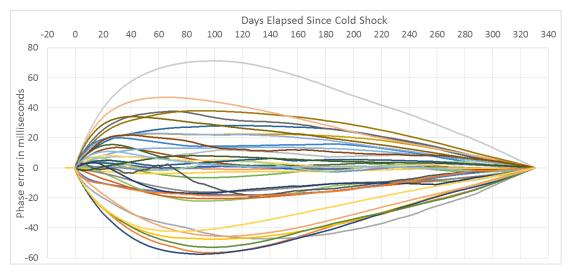
The figure to the left shows Seascans tested in a temperature chamber at 2°C over an 11 month simulated deployment. Offset between each clock and GPS is measured once per minute. At the end of the experiment we apply a linear clock drift correction based on end-points, as is done in an actual OBS experiment. This figure shows the difference between the drift-corrected time and the true time as measured by the GPS clock. We use these tests to select the best performing clocks.
