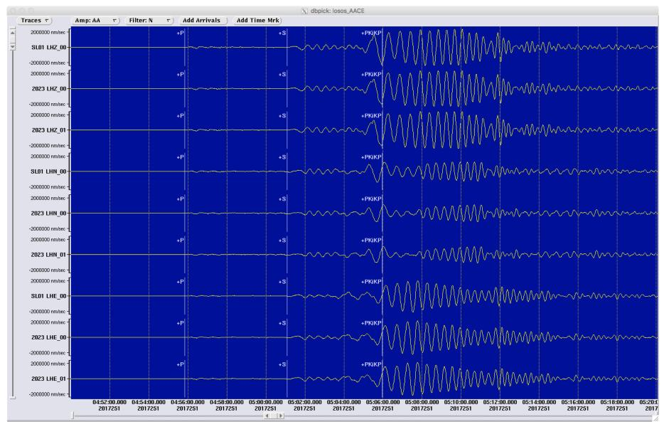
Ground motion from the September 08, 2017 Mw 8.2 Mexico earthquake recorded by our reference sensor (station SL01), and 2 Guralp stations (2023\_00, and 2023\_01). Epicentral distance is 33°. Data are unfiltered.
