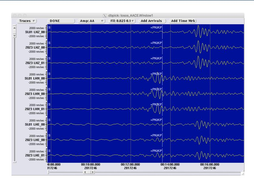
Ground motion from the September 02, 2017 Mw 5.3 Eastern Idaho earthquake recorded by our reference sensor (station SL01), and 2 Guralp stations (2023\_00, and 2023\_01). Epicentral distance is ~30°, and the back-azimuth is 286°, so the the E-W and N-S components are approximately radial and transverse, respectively. The three stations show good coherence for Love and Rayleigh waves arrivals in the frequency band (0.025–0.1 Hz).
