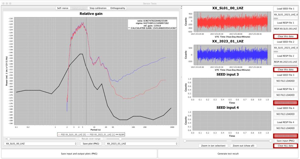
Calibration of Guralp CMG-3T seismometer S/N T3G38 relative to WHOI's Nanometrics Trillium 240 reference sensor. The calibration procedure, from USGS Albuquerque, compares power spectral density levels in the microseismic band. This particular Guralp sensor shows a calculated sensitivity of 1546 V/m/s. The factory-specified sensitivity for this channel was 1490 V/m/s, an ~4% change.
