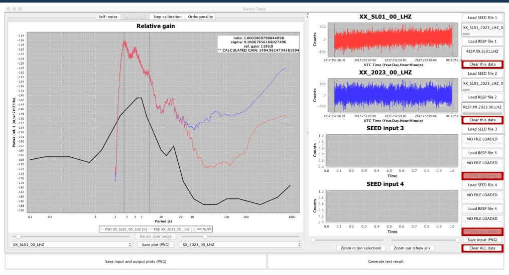
Calibration of Guralp CMG-3T seismometer S/N T3G92 relative to WHOI's Nanometrics Trillium 240 reference sensor. The calibration procedure, from USGS Albuquerque, compares power spectral density levels in the microseismic band. This particular Guralp sensor shows a calculated sensitivity of 1495 V/m/s. The factory-specified sensitivity for this channel was 1494 V/m/s.
