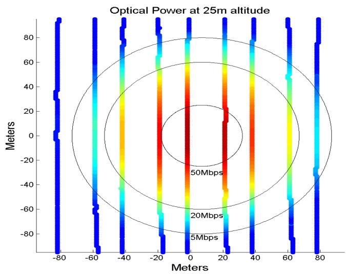
Optical modem power at 25 m altitude measured with the Sentry AUV. Circles of constant data rate are shown and labeled. These define the size of the loiter circle that an AUV needs to maintain to ensure the given data rate.
