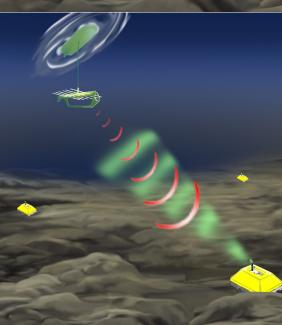
The optical modem is a versatile instrument that can be used from a variety of platforms. In addition to using an AUV (top left), the modem can be lowered on a ship's standard CTD wire to within ~100 m of the OBS (top right). Dynamic positioning is not necessary. Finally, Liquid Robotics<sup>®</sup> is now developing a winch system for their glider that will be capable of lowering the modem to ~150 m depth while providing 10 W of power and 10 Mbits/s Ethernet at the end of the wire.
