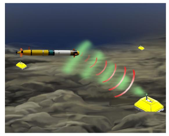
Accurate timing is critical for earthquake location but OBS lack GPS timing. The optical link will also allow measurement of the offset of the OBS clock relative to a GPS-synchronized time signal carried by the AUV to a precision of ~1 microsecond.
