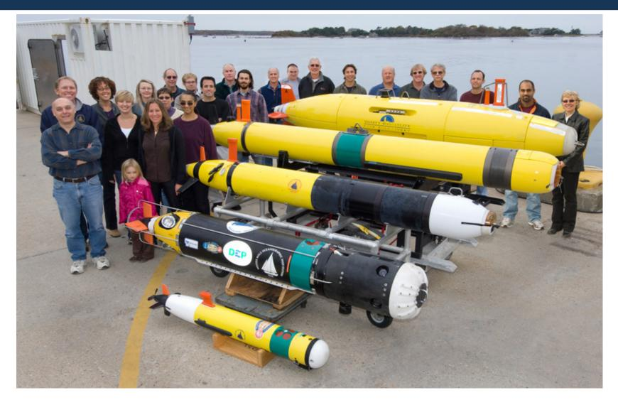
The REMUS (Remote Environmental Monitoring UnitS) family of autonomous underwater vehicles (AUVs). From front to back: REMUS-100, REMUS Tunnel Inspection Vehicle, REMUS-600, REMUS-3000, and a REMUS-6000. The numbers indicate maximum operating depth in meters.
