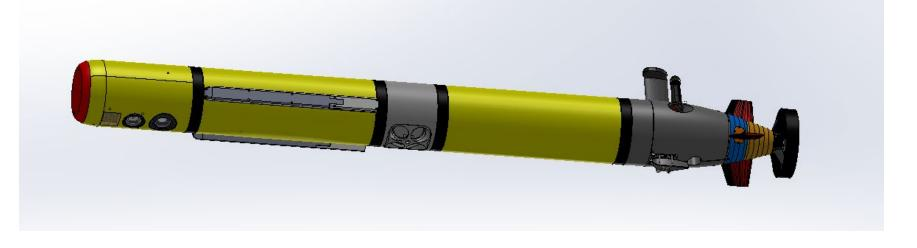
CAD drawings of how the optical modem will be mounted on the belly of the REMUS 600
