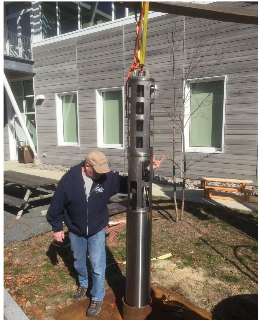
Tim Kane, watched by Jeff O' Brien (left) and Keith von der Heydt (right) guides the BIP (Bottom Instrument Package) into the borehole just outside the OBS Lab.
