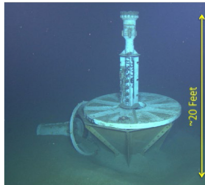
View of the seafloor component of the ACORK (Advanced Circulation Obviation Retrofit Kit) installed at Hole U1364A in 2010.
