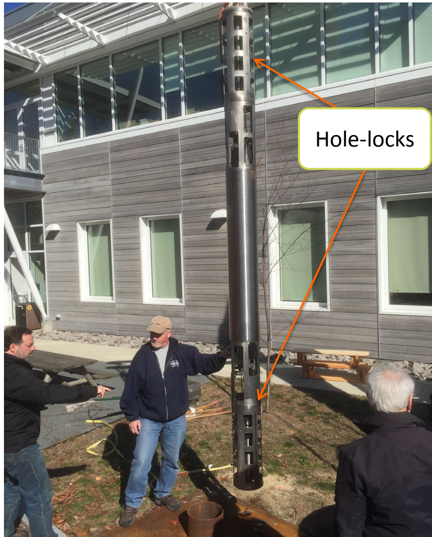
Tim Kane, watched by Jeff O' Brien (left) and Keith von der Heydt (right) guides the BIP (Bottom Instrument Package) into the borehole just outside the OBS Lab.
