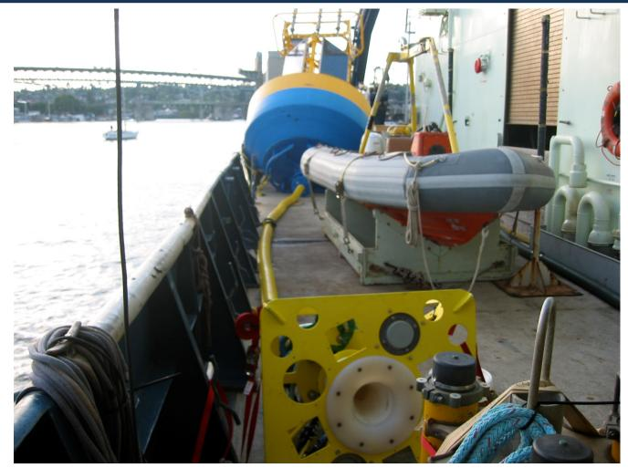
A 10 m chain-urethane composite around which are coiled 12 conductors connects two acoustic-modem transducers mounted on an aluminum plate to electronics in the surface buoy. The purpose of this component is to protect the conductors from the bending strains produced by the motion of the buoy in severe sea states.
