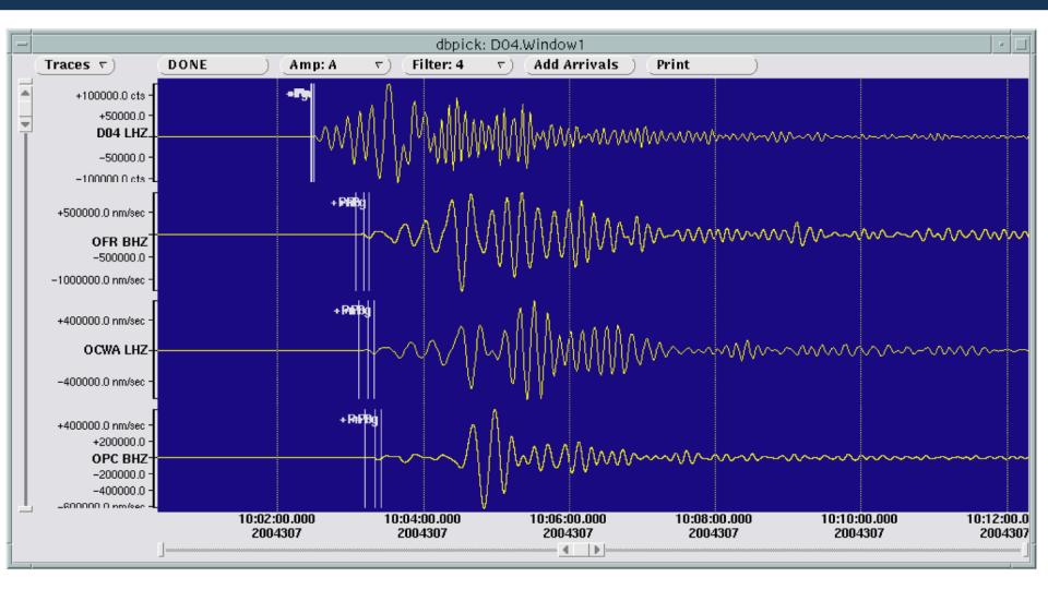
Vertical-component seismograms for the 2004-11-02 Mw 6.6 Vancouver Island event. Station D04 is the acoustically-linked WHOI OBS at an epicentral distance of ~0.8° from the epicenter. These data were telemetered to shore in near real-time. Seismograms from 3 nearby land stations are shown for comparison, and are located at distances of 3.2° (OFA), 3.5° (OCWA), and 3.8° (OPC).
