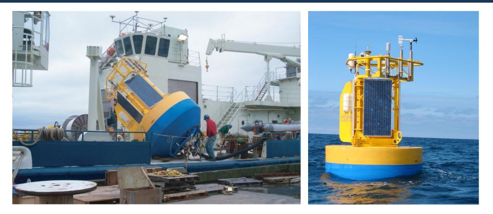
The surface buoy consisted of a 2.7-m diameter Surlyn float with 6800 kg of net buoyancy. The aluminum structure mounted atop the float includes a tower for securing instruments and antennas as well as four 150-watt solar panels. The buoy's average 5 watt/day power consumption was provided by a rechargeable bank of lead-acid cells augmented by a backup battery capable of providing power for up to three months.
