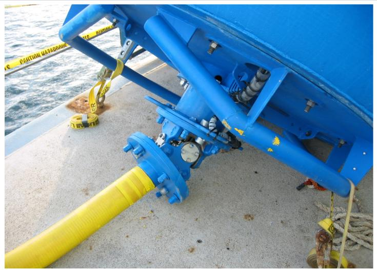
Unique features of the buoy and mooring include a universal joint between the buoy and the mooring that provides for up to about 60 degrees of motion in two planes. A central hole in the universal provides an unbending pathway for conductors that pass through the universal.
