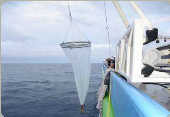
Figure 3. The Indian Ocean Standard Net (IOSN) is the one of the original nets used in the International Indian Ocean Expedition in the 1960s. This one being deployed from the RV Investigator on the 110°E line is a replica allowing for interesting comparisons of zooplankton biomass and composition across the decades since the 1960s. Photo: Micheline Jenner AM
