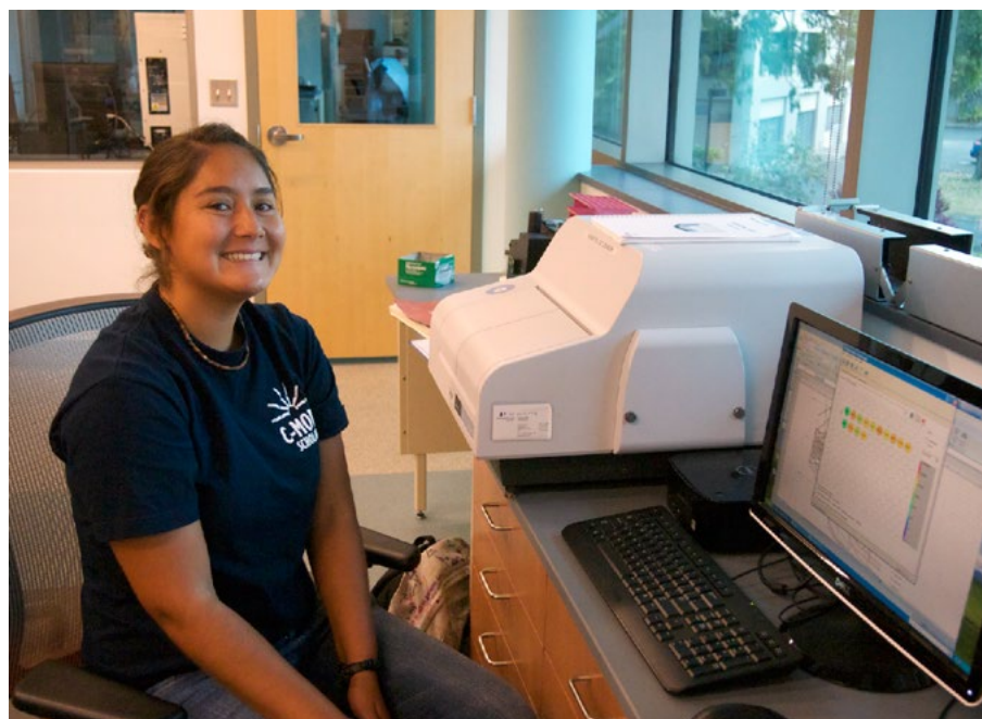
Figure 1. Kirena Clah reading chlorophyll autofluorescence on a plate reader as a measure of algal culture health after inoculating the cultures with the purified bacterium.
