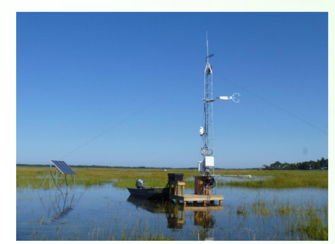
Fig.3 : Measurement set up (Campbell Sci. EC200 closed path system) at PIE during a spring tide (z=4.16m at low tide)
