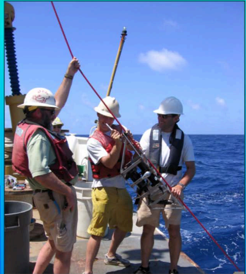
Deployment of fluorometer on an ATLAS mooring
