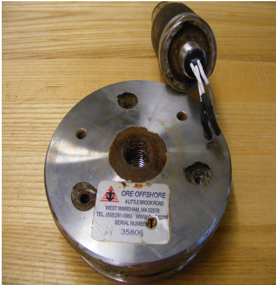
Severe corrosion identified on baseplate and penetrator
