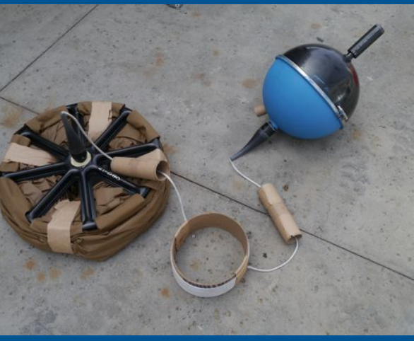
Lagrangian drifters measure near-surface ocean currents, atmospheric pressure, sea surface temperature and sea surface salinity
