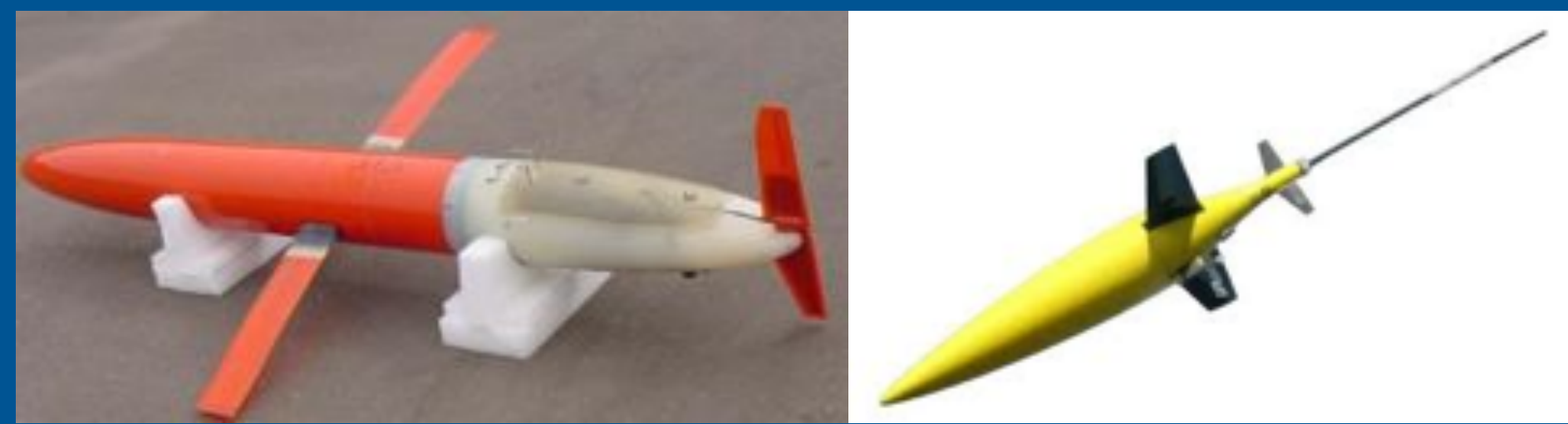
Long term endurance gliders Spray (left) and Seaglider (right) measure subsurface temperature and salinity structure.
