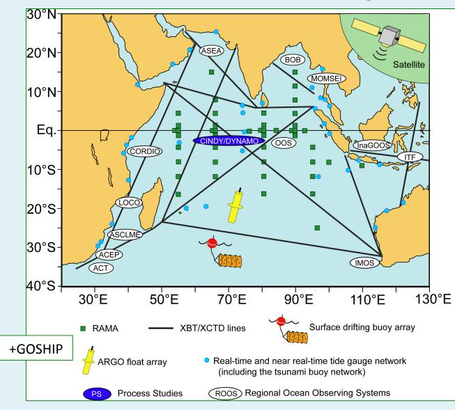
A network of in situ & satellite components designed to provide sustained high-quality oceanographic and marine meteorological measurements to support knowledge based decision-making through improved scientific understanding, weather and climate forecasts, and environmental assessments for the benefit of society.
