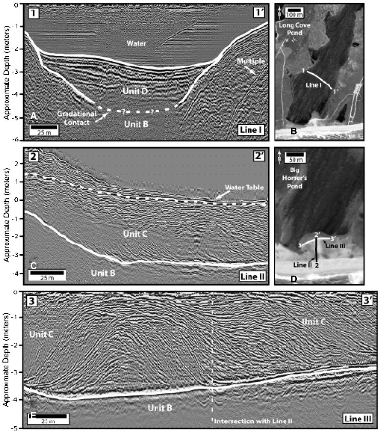
**Fig. 4.** GPR profiles with sedimentary units identified. Vertical scale is referenced to each pond's still water level. Box A: radargram from Long Cove Pond (location of line is indicated in box B) taken through the water column. Box C is a radargram from Big Homer's Pond taken on land and topographically corrected. Location of line is given in Box D. Box E is a radargram from Big Homer's Pond taken on land and topographically corrected (profile is flat). Location of line is given in box D.
