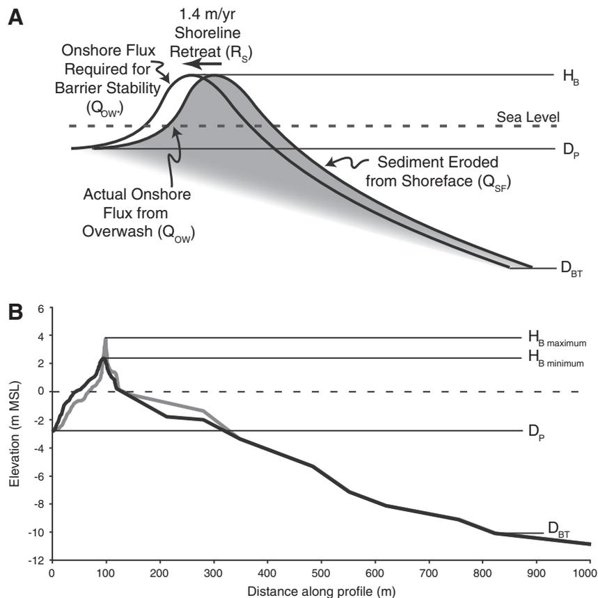
**Fig. 9.** (A) Schematic depicting the amount of onshore sediment flux,  $Q_{OW^*}$ , required to maintain a stable barrier width during shoreline retreat,  $R_s$ , related to the actual amount of onshore sediment flux from overwash,  $Q_{OW}$ . Heights used in the estimation are the pond depth,  $D_P$ , barrier toe depth,  $D_{BT}$ , and barrier height,  $H_B$ . (B) Heights used in estimation from minimum and maximum from example profiles at Big Homer's Pond.
