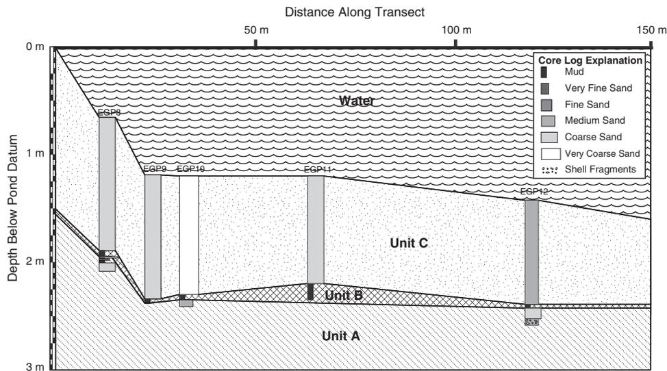
Fig. 5. Stratigraphic section of five cores from Edgartown Great Pond showing Units A through C. Cores used in the profile are labeled in Fig. 3. The distance along transect goes from south (0 m) to north (150 m).
